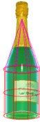
Figure 1: The haptic model of a bottle consists of a cylinder in combination with a cone. [2]
